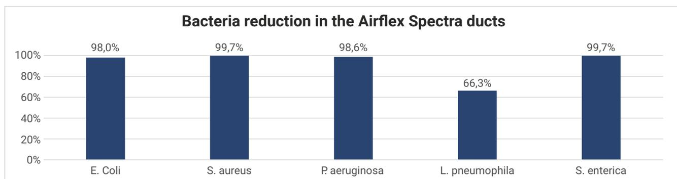
Test of antibacterial properties of the polymer material in a 24 h test. The graph shows the bacteria reduction degree after 24 h contact with the Airflex Spectra sample.
